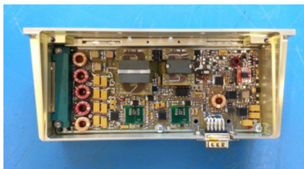
Figure 4. Above: The Electrical Model Readout Electronic Power Supply Unit. Right: The Electrical Model Power Mechanism Control Unit.
