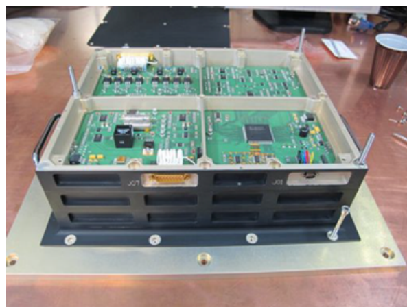
Figure 4. Above: The Electrical Model Readout Electronic Power Supply Unit. Right: The Electrical Model Power Mechanism Control Unit.
