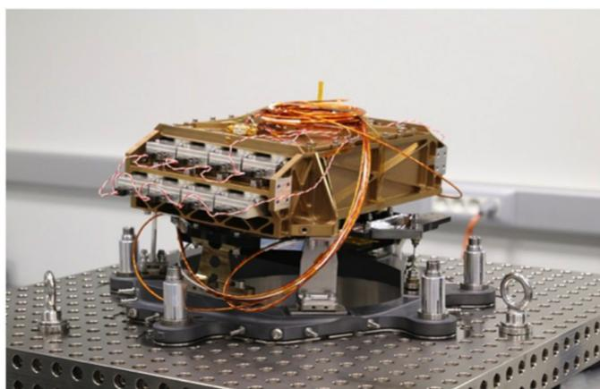
Figure 4. Left: The **structure and thermal model (STM)** of the optical assembly at AIT. Right: a model of the STM of the focal plane.
