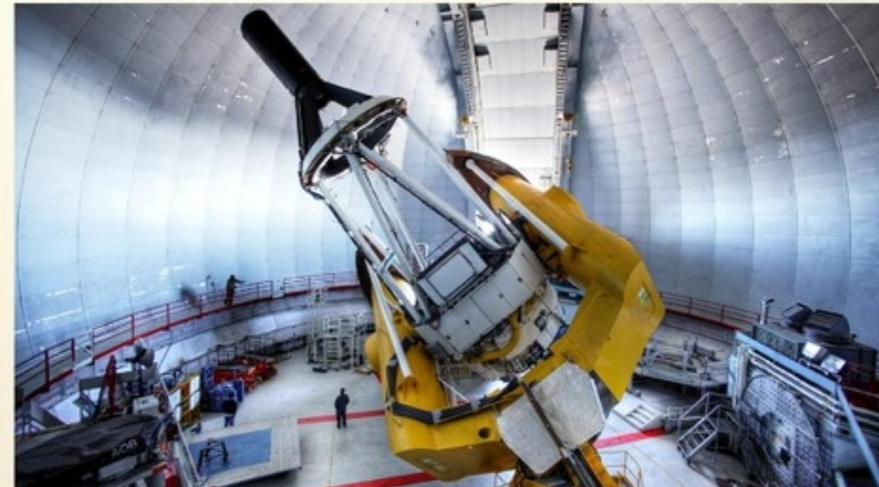
Equatorial mount with prime focus cage
