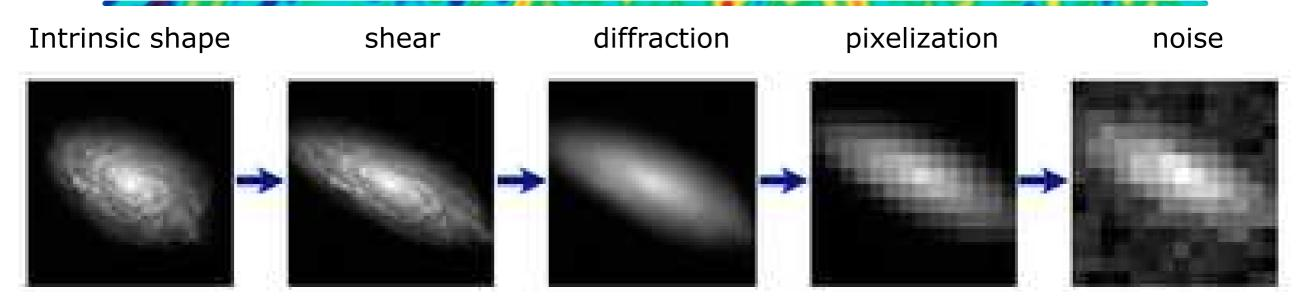
$$\tilde{e} = \gamma + e_{\text{intrinsic}} + c + m (\gamma + e_{\text{intrinsic}}) + q (\gamma + e_{\text{intrinsic}})^2 + o(\gamma^3, e^3)$$
