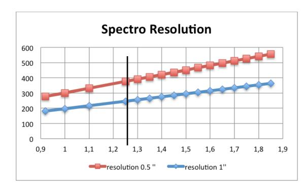
R-NISP-P-0XX The NISP spectrometric channel spectral effective resolution R considering a reference 0.5" diameter source shall be  $R=\lambda/\Delta\lambda > 260$  over the full B-band spectral range.
